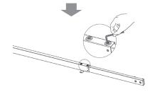
Attach the telescopic crossbar to the lifting columns as shown by using the screws identified in the illustration.
